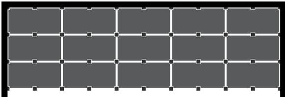
Diagrams depict carpet tile Monolithic installations only. For other installation methods, ensure tabs are placed on all tile corners and an extra tab in the long direction of 18 in x 36 in tiles. Use half tabs at walls.
